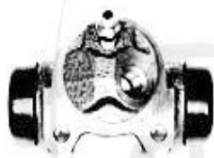
1. RBZ 177 links/left System: Bendix Ø 17,46 mm > 1986 - 4x4
